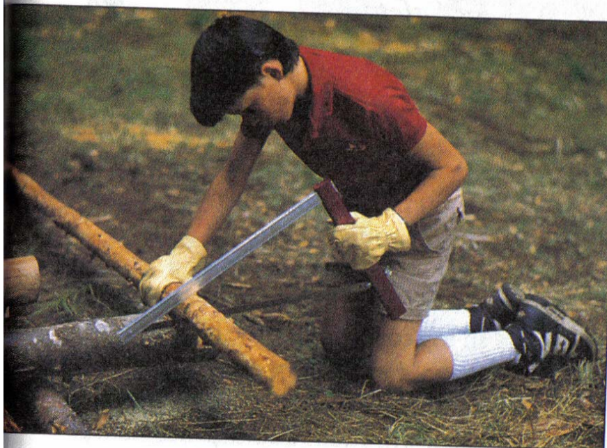
Place the wood you are cutting so that the cut end falls free of the support.
